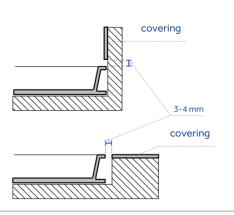
Position the shower tray paying attention to the thickness of the covering (or to the floor thickness in case of recessed installation) and leaving a gap of 3-4 mm.
