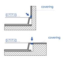
Verify the right horizontal positioning by means of a spirit level.
