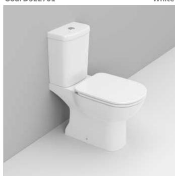
Universal outlet close coupled, for assembly with CC cistern 4,5 L. Necessary equipment: cistern, mechanism, seat and cover, outlet bend in case of vertical installation. Fixation set included.
