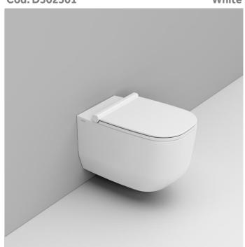
Wall hung bowl, 4,5 L flush, due to rimless system and interior surface design. For assembly with suitable wall mounted chair brackets. Including fixation kit for hidden attachment. To be completed with seat and cover.
